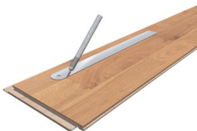
Cut through the lacquer layer in the joints around the strip. Use a straight edge.
