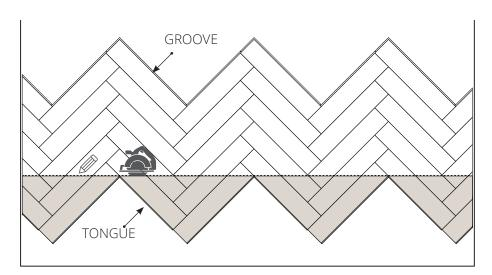
**10.** Push the trimmed floor planks toward the wall, ensuring there's a 10 mm gap between the planks and the wall.
