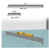
that the subfloor is flat and level over measured lengths of 2 m and 0.25 m. If any unevenness exceeds 3 mm over 2 m and 1 mm over 0.2 m, the floor must be levelled first.
