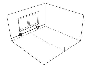
**2.** When laying the first row, pay attention so that the sides of the planks are perfectly aligned. Place the first row right in the center of the room, so that the distance from A and B is identical.
