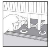
Installation around radiators. Drill holes 5-10mm bigger than the diameter of the pipes. Glue together the block behind the pipes.
