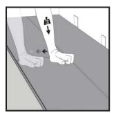
Press down with your hand or tap lightly with a rubber mallet on the tile you just installed.
