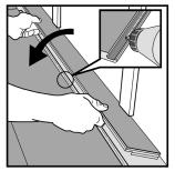
Cut off locking element using a chisel, apply PVC adhesive to the adjusted strip and press the tiles together horizontally. If necessary, place spacers between the final plank and the wall while the adhesive hardens.
