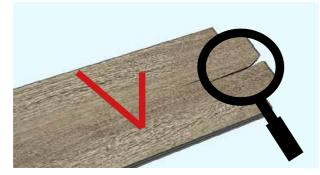
You shall inspect every floorboard carefully, before installing it to avoid any damaged or faulty boards are being installed. It is always easier to rectify faults if they are discovered early. It is important to always inspect the product during installation. If faulty products are discovered regarding, for example, appearance or other design elements that do not correspond to what is described in the product sheet, it is important that a complaint is made before you install the floor.
