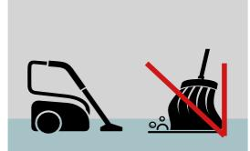
Always vacuum-clean the subfloor before installing any underlay and or floorboards, to remove any debris on the surface.
