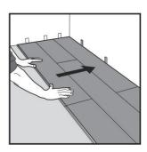
After 2-3 rows. Adjust the distance to the front wall by positioning a distance of 1/2".
