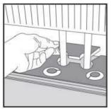
Installation around radiators. Drill holes 1/2" bigger than the diameter of the pipes. Glue together the block behind the pipes.
