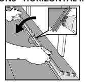
Cut off locking element using a chisel, apply Landobond (ID# 710225) adhesive to the adjusted strip and press the tiles together horizontally. If necessary, place spacers between the final plank and the wall while the adhesive hardens.
