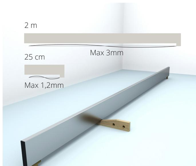
Without exception check that the subfloor is flat and level over measured lengths of 2m and 0.25m. If any unevenness exceeds +/- 3mm over 2m and +/- 1.2mm over 0.25m, the floor must be levelled prior to installation of the Aware floor. Kährs also accepts a measuring length of 1 m. The tolerance in this case is +/- 2mm.
