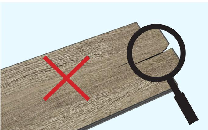
**Note** Some decors may contain elements that may be perceived as deviating for an individual board, but which on an installed floor surface is an approved and conscious design element. Always make sure that inspection and installation takes place with good lighting conditions!
