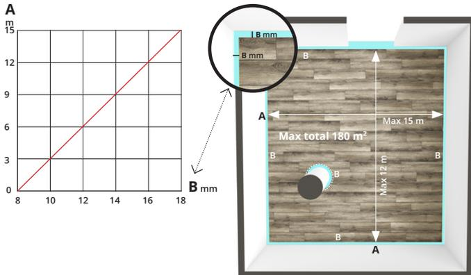
The size of the movement joint in mm is calculated using the formula:  $2\text{mm} \times 3\text{-meter floor area}$ . The size of the movement joint should never be less than 8mm. Remember to remove the spacers after installation is done and complete.
