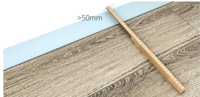
When installing the Aware floor, it is easier if the installation is started at the long side that has the most doors. If there are doors on the short sides of the room, it is also easiest to start a new row of boards from that side. The boards can be laid both from the left and right and backwards. If the floor width and length exceed the specified maximum joint dimensions, the floor must be divided by an expansion joint.
