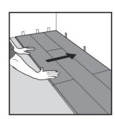
After 2-3 rows. Adjust the distance to the front wall by positioning a distance of 5-10mm.
