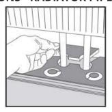
Installation around radiators. Drill holes 5-10mm bigger than the diameter of the pipes. Glue together the block behind the pipes.
