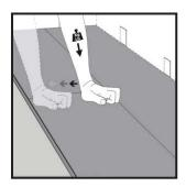
Press down with your hand or tap lightly with a rubber mallet on the tile you just installed.
