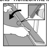
Cut off locking element using a chisel, apply PVC adhesive to the adjusted strip and press the tiles together horizontally. If necessary, place spacers between the final plank and the wall while the adhesive hardens.
