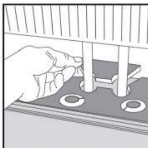
Installation around radiators. Drill holes 10 mm bigger than the diameter of the pipes. Glue together the block behind the pipes.
