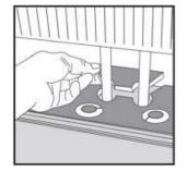
Installation around radiators. Drill holes 1/2" bigger than the diameter of the pipes. Glue together the block behind the pipes.
