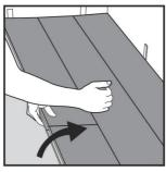
Separate the whole row by carefully lifting up and releasing the whole row. Fold up and release the whole long side.
