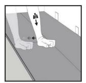
Press down with your hand or tap lightly with a Kährs handblock on the tile you just installed.
