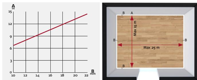
Note that the dimensions of the skirting board must never determine the size of movement joints. With large floor areas, the skirting board must therefore be selected on the basis of the required size for the expansion joint and not vice versa.
