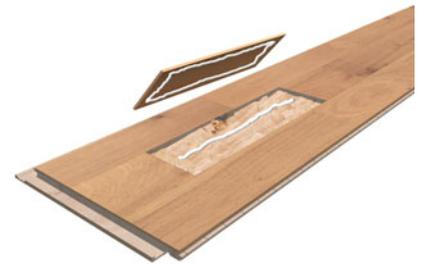
Select and fit a replacement strip. Fill the cavity with epoxy and press the strip down.
