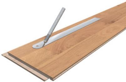
Cut through the acrylic finish layer in the joints around the strip. Use a straight edge.
