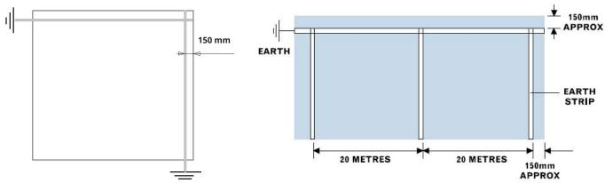
Figure 1. Earthing strip layout small area, less than 10 m x 10 m.
