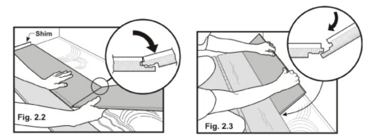
2.3 Use cut off from first row to start second row (Fig. 2.3). With groove side facing first row, hold board at approximate 45° angle and press inward, completely engaging long side joint. Ensure end joint stagger from row to row is a minimum of 20" for 14mm and 15mm and a minimum of 12" for 7mm and 10mm flooring.
